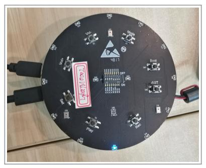
Figure 2-6. The LED Light on ESP32-LyraTD-MSC
