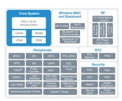
ESP32-C3 Block Diagram
