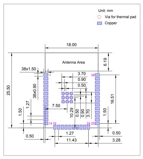
Figure 6: Recommended PCB Land Pattern of ESP32-SOLO-1
