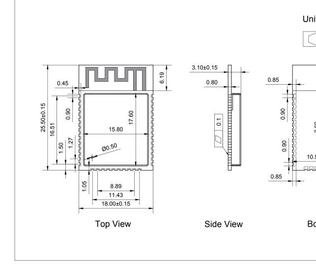
Figure 5: Physical Dimensions of ESP32-SOLO-1
