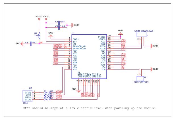
Figure 4: ESP32-SOLO-1 Peripheral Schematics
