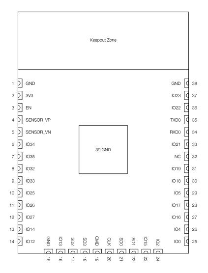
Figure 1: ESP32-SOLO-1 Pin Layout (Top View)
