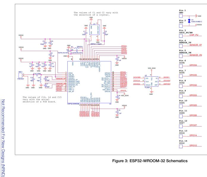
Figure 3: ESP32-WROOM-32 Schematics
