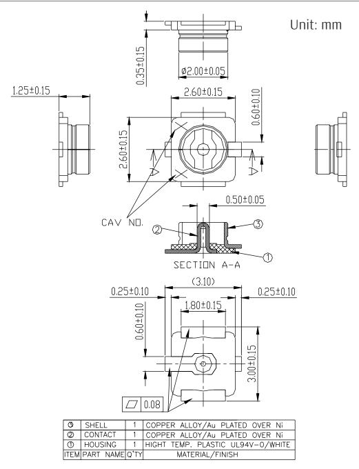
Figure 8: U.FL Connector Dimensions
