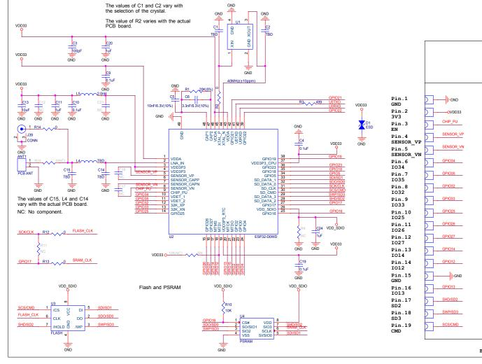
Figure 4: Schematics of ESP32-WROVER-IB
