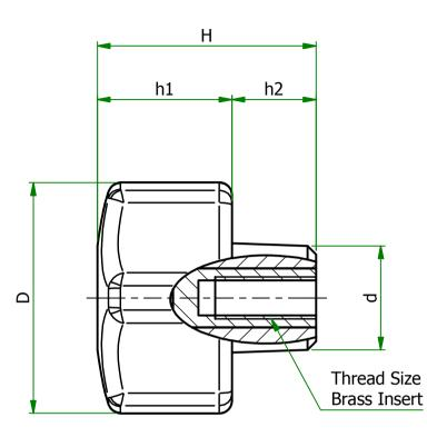
NOTE: INSERT MATERIAL: BRASS INNER MOULDING: PP OVER MOULDING: TPE
