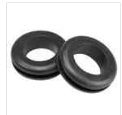
Open Hole Grommet, Black, TPV, .970 in ID, 1.500 in OD, .313 in Thick, 1.240 in Hole Dia
