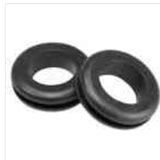
Open Hole Grommet, Black, TPV, .500 in ID, .954 in OD, .280 in Thick, .748 in Hole Dia
