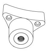
**Note:** Threaded parts must accept 2A GO gage. Per current fastener industry practice, if form, fit, and function are achieved, parts may accept 2A NO GO.
