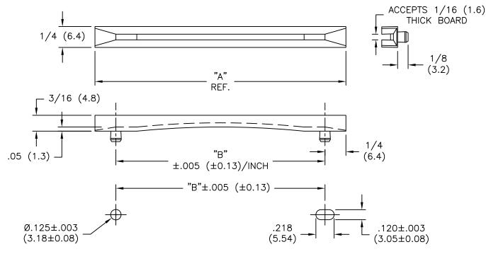
RECOMMENDED MOUNTING HOLES IN 1/16" (1.6) NOMINAL THICK PANEL
