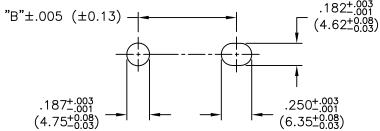
RECOMMENDED MOUNTING HOLES PANEL THICKNESS: .047-.090 (1.2-2.3)
