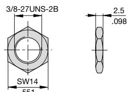
This is a metric design and millimeter dimensions take precedence ( $\frac{\text{mm}}{\text{inch}}$ )
