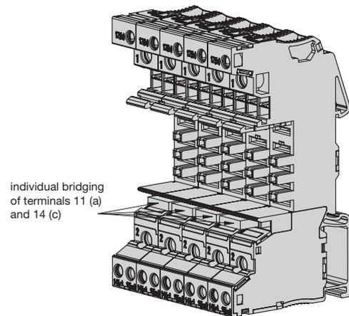
**Parallel connection of auxiliary contacts**
