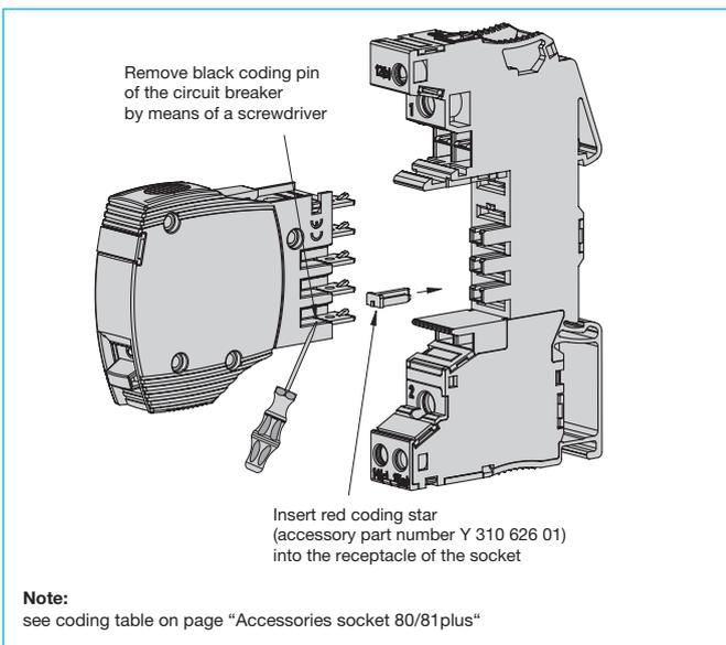
**Replacing a circuit breaker**
