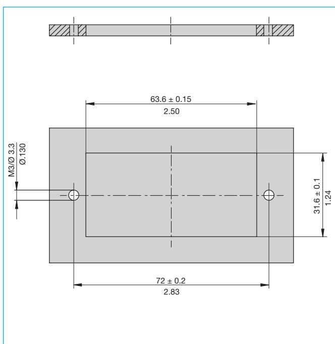
This is a metric design and millimeter dimensions take precedence ( $\frac{\text{mm}}{\text{inch}}$ )
