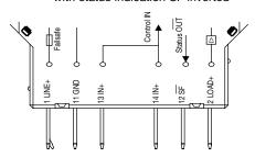
Standard condition: SF 0V = OK Fault condition: SF +24V
