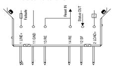
Standard condition: SF + 24V = OKFault condition: SF 0V
