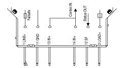
Standard condition: SF+24V = OK Fault condition: SF 0V
