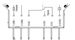
Standard condition: SC/SO closed, SC-SI open Fault condition: SC/SO open, SC-SI closed
