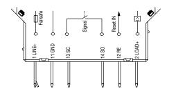
Standard condition: SC/SO closed Fault condition: SC/SO open
