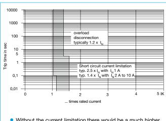
• Without the current limitation there would be a much higher overcurrent in the event of an overload or short circuit.
