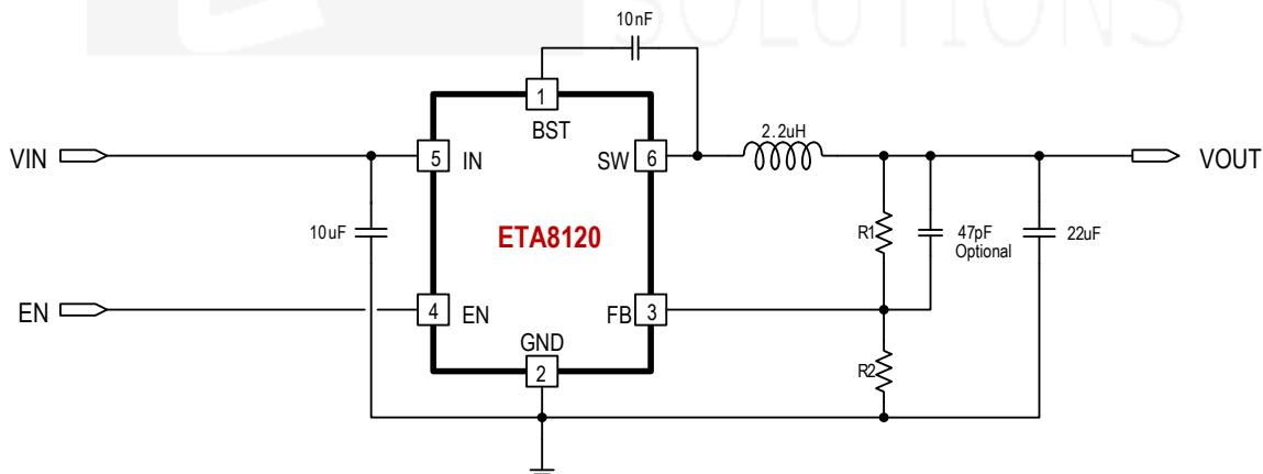
$$V_{out} = \frac{R_1+R_2}{R_2} \times 0.6(V)$$
