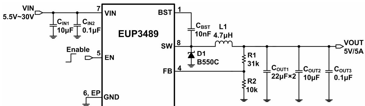
Figure 1. 5V Application Circuit
