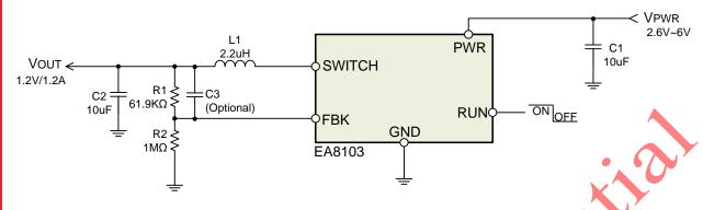
Figure 2. Typical application circuit diagram
