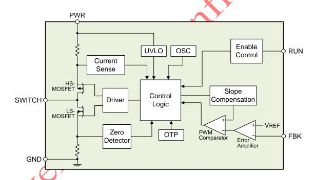
Figure 1. EA8103 internal function block diagram
