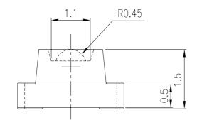
For reflow soldering (propose)
