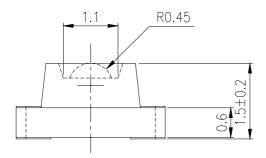
For reflow soldering (propose)
