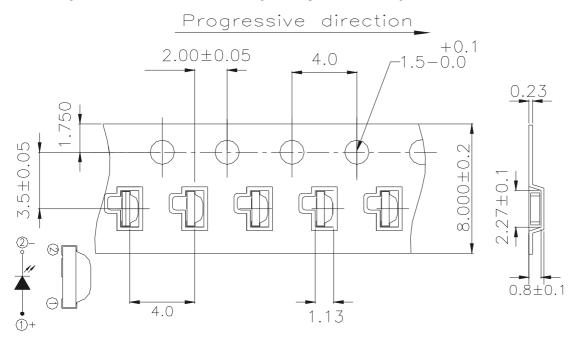
Note: The tolerances unless mentioned is  $\pm 0.1$  mm ,Unit = mm **Moisture Resistant Packaging**
