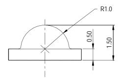
For reflow soldering (propose)
