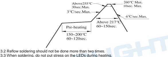
3.4 After soldering, do not warp the circuit board.
