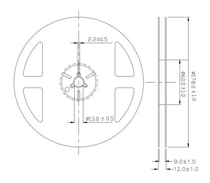
**Note:** The tolerances unless mentioned are  $\pm 0.1$ , unit = mm.
