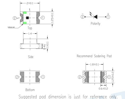
Please modify the pad dimension based on individual need. Note: Tolerances unless mentioned  $\pm 0.1$ mm. Unit = mm
