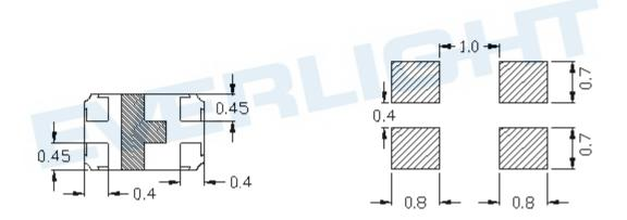
**Note:** The tolerances unless mentioned are  $\pm 0.1$  mm ,Unit = mm
