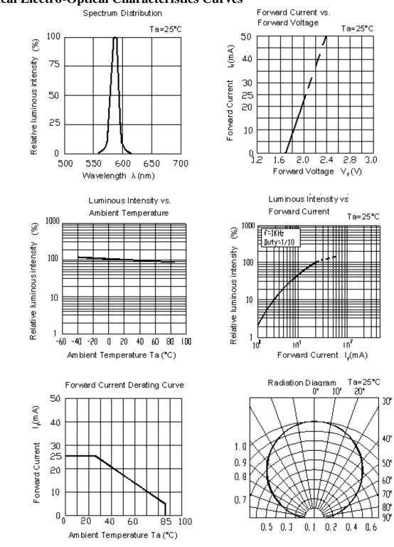
**Typical Electro-Optical Characteristics Curves**
