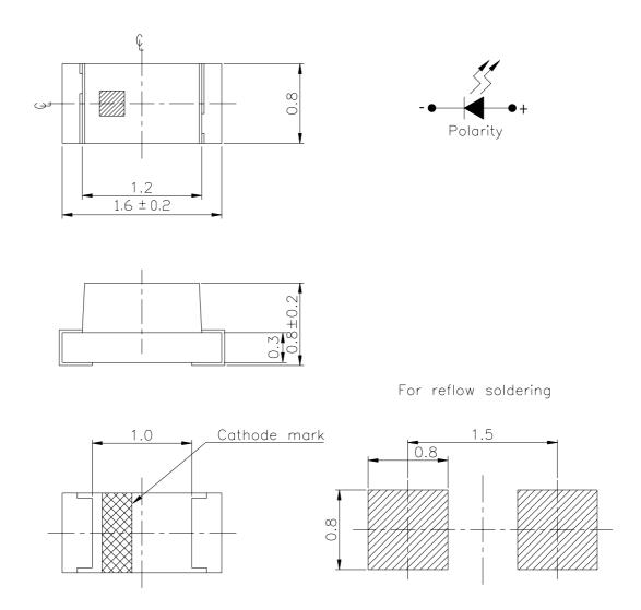
**Note:** The tolerances unless mentioned are  $\pm 0.1$ , unit = mm.
