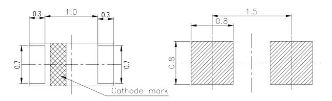
**Note:** The tolerances unless mentioned is  $\pm 0.1$ mm ,Unit = mm
