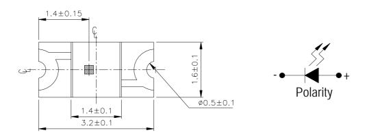
For reflow soldering (propose)
