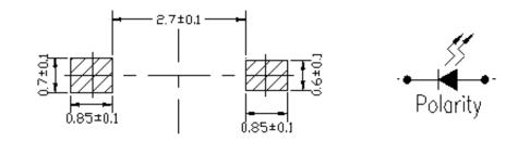
Note: The tolerances unless mentioned are  $\pm 0.1$ , unit=mm.
