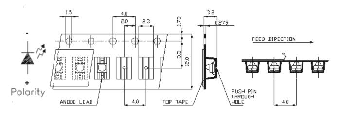
Note: The tolerances unless mentioned are ±0.1, unit=mm.
