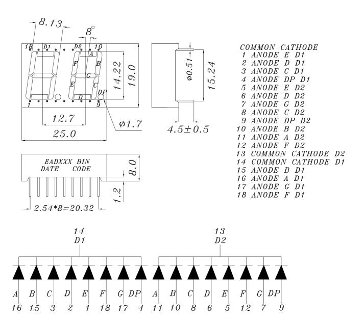
Note: Tolerances unless mentioned ±0.25mm. Unit = mm
