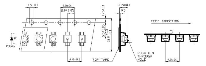
Note: The tolerances unless mentioned are ±0.1, unit=mm.
