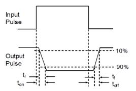
Figure 10. Switching Time Test Circuit & Waveforms
