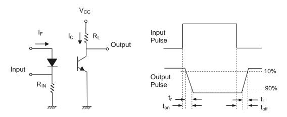
Figure 7. Switching Time Test Circuit & Waveforms
