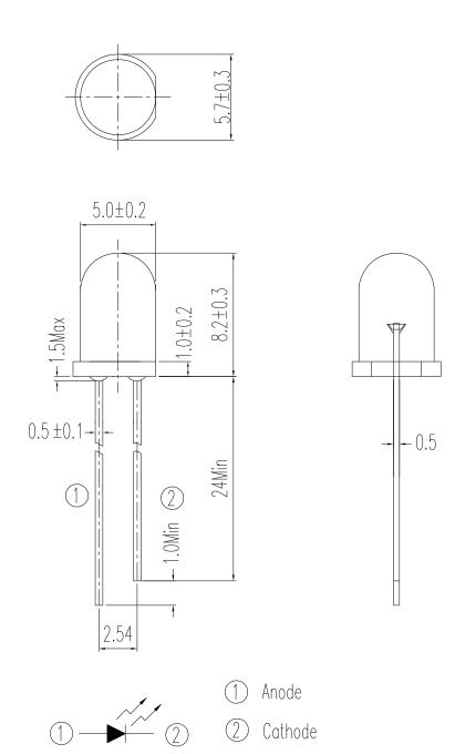
Note: Tolerances unless dimensions ±0.25mm
