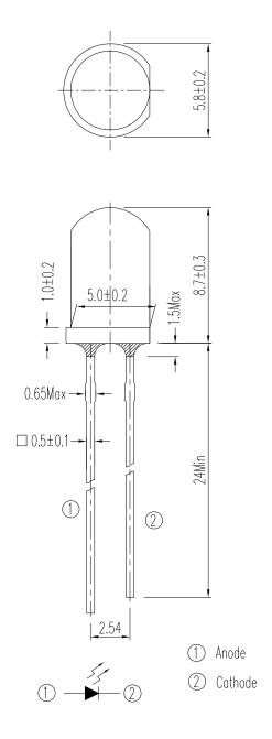
Note: Tolerances unless dimensions ±0.25mm
