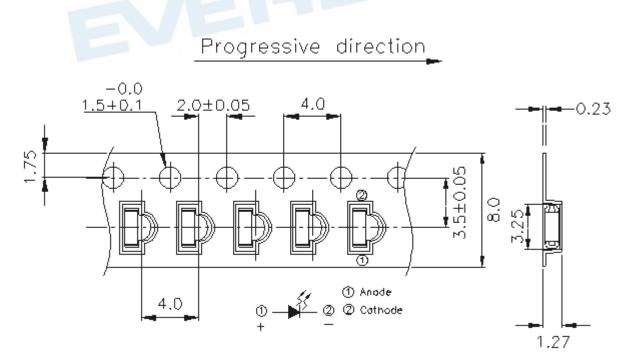
Note: The tolerances unless mentioned are ±0.1mm, unit: mm
