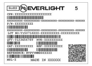
CPN: Customer's Production Number P/N : Production Number LOT No: Lot Number QTY: Packing Quantity HUE: Peak Wavelength CAT: Ranks REF: Reference MSL-X: MSL Level Made In: Manufacture place
