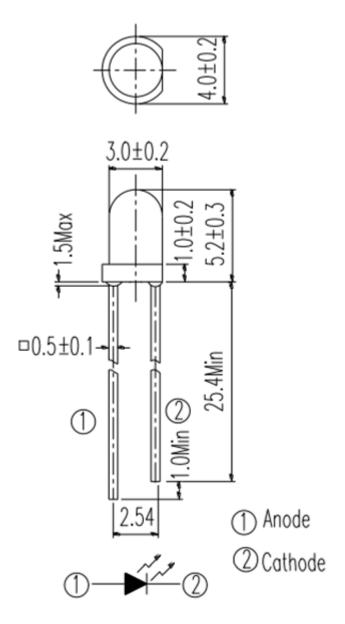
Note: Tolerances unless dimensions ±0.25mm
