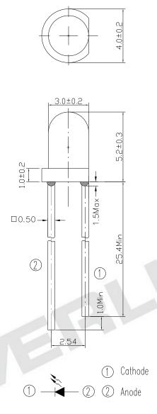
Note: Tolerances unless dimensions ±0.25mm
