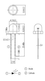
Note: Tolerances unless dimensions ±0.25mm
