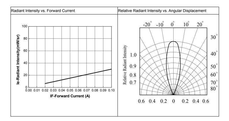
DATASHEET 5.0mm Infrared LED IR323
