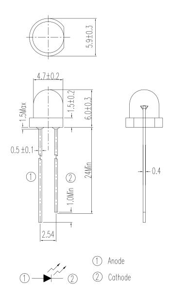
Note: Tolerances unless dimensions ±0.25mm
