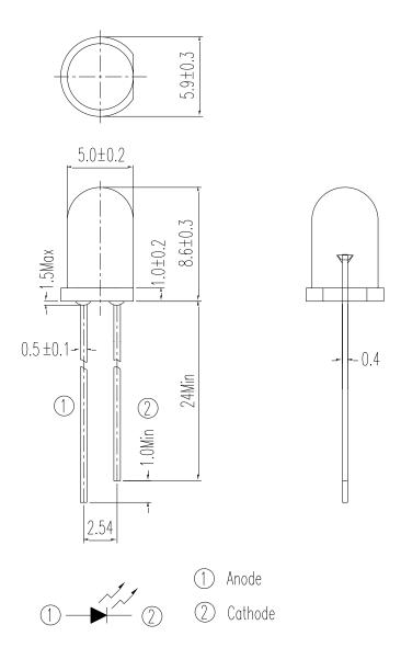
Note: Tolerances unless dimensions ±0.25mm
