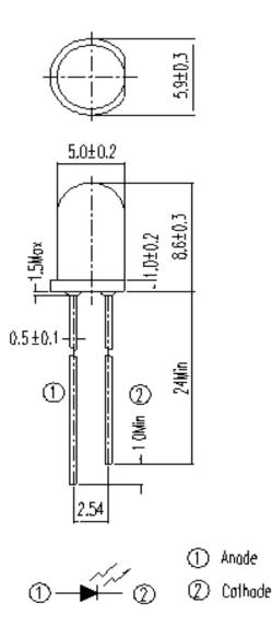
Note: Tolerances unless dimensions ±0.25mm
