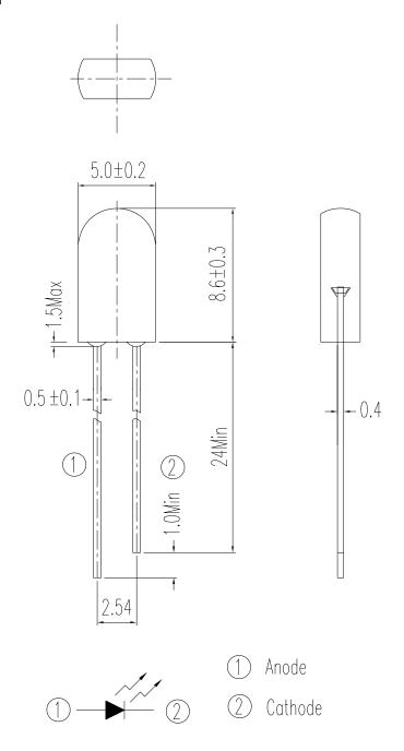
Note: Tolerances unless dimensions ±0.25mm
