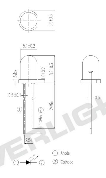
Note: Tolerances unless dimensions ±0.25mm
