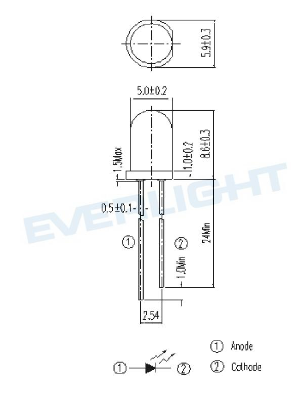
Note: Tolerances unless dimensions ±0.25mm
