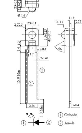
Notes: 1. All dimensions are in millimeters 2. Tolerances unless dimensions ±0.3 mm
