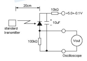
Fig.-3 Measuring System
