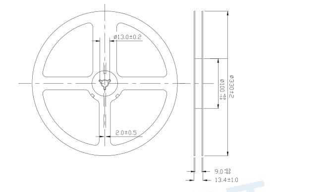
**Note:** The tolerances unless mentioned is  $\pm 0.1$ mm ,Unit = mm **Carrier Tape Dimensions :**( **Quantity: 3000pcs/reel**)
